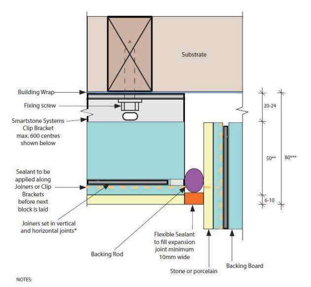
\* Maximum space between joiners or joiners & clips to be 20mm. Care must be taken to ensure sealant is applied along all extrusions and clips, and that particular care is taken to ensure adequate sealant applied to ensure spaces are filled.
