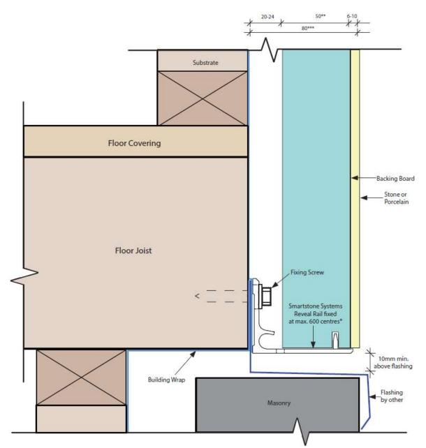
NOTES: \* Care must be taken to ensure sealant is applied along all extrusions and clips, and that particular care is taken to ensure adequate sealant applied to ensure spaces are filled.
