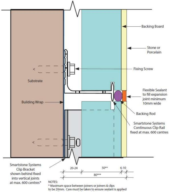
to be 20mm. Care must be taken to ensure sealant is applied along all extrusions and clips, and that particular care is taken to ensure adequate sealant applied to ensure spaces are filled.
